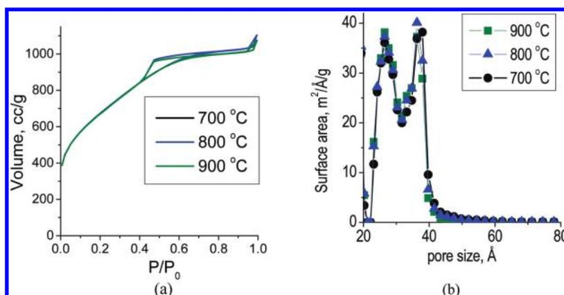
Figure 4. Porosity of CDC samples: (a)  $\text{N}_2$  sorption isotherms recorded at 77 K on mesoporous CDC samples and (b) pore size distribution of aligned mesopores calculated using slit-pore DFT model.
