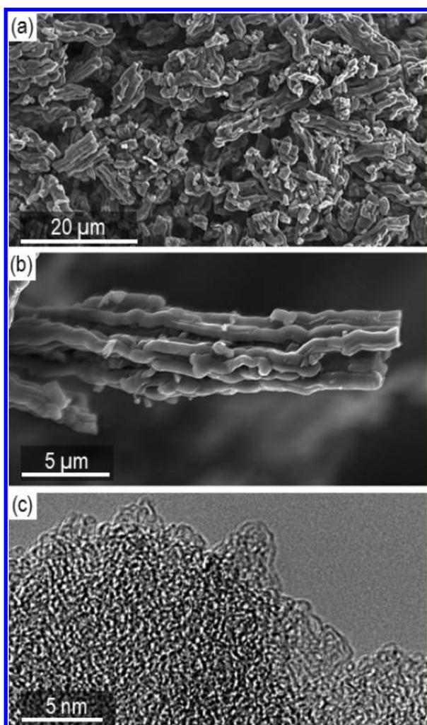
Figure 2. Electron microscopy of CDC samples: (a, b) SEM micrographs recorded at different magnification and showing the morphology of the produced particles; (c) high resolution TEM micrograph showing the microstructure of CDC.
