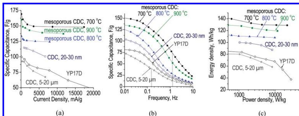
**Figure 7.** Electrochemical characterization of CDC with aligned mesopores produced at 700, 800, and 900 °C in comparison to that of activated carbon commonly used in commercial EDLC (YP17D) and CDC produced from micrometer-size and nanosize SiC powder at 900 °C: (a) capacitance retention with current density, (b) frequency response of capacitance, and (c) Ragone plot of energy density vs power density.
