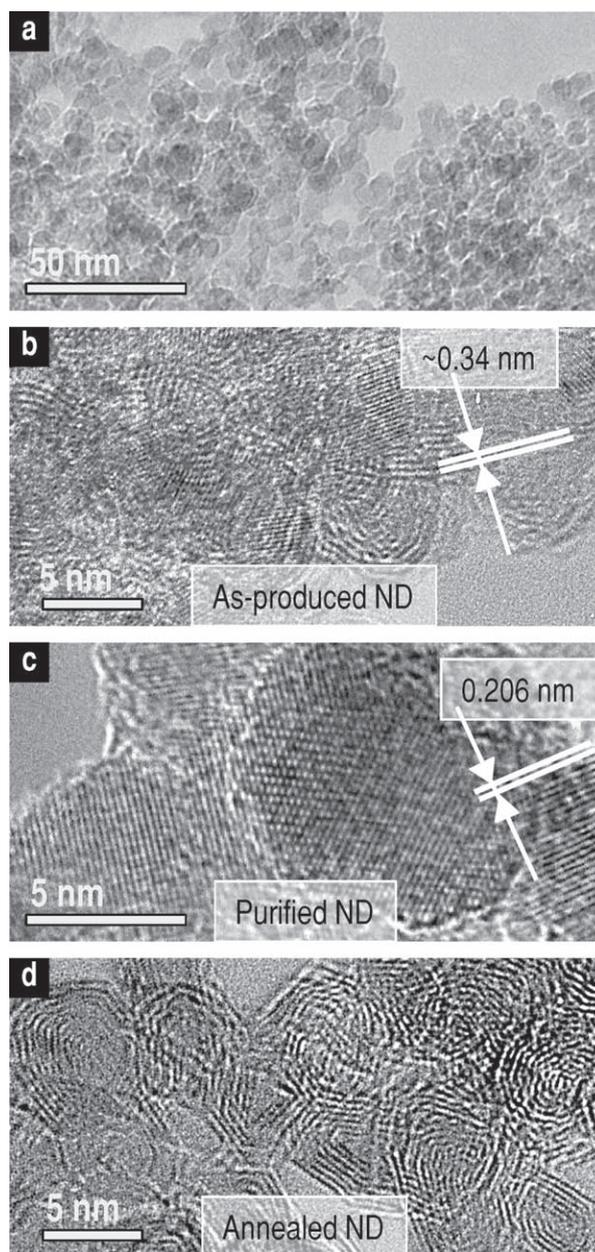
**Figure 2.** TEM images of the ND samples: a) low-resolution micrograph of ND powder, b) ND soot, c) purified ND, d) annealed ND (OLC)
