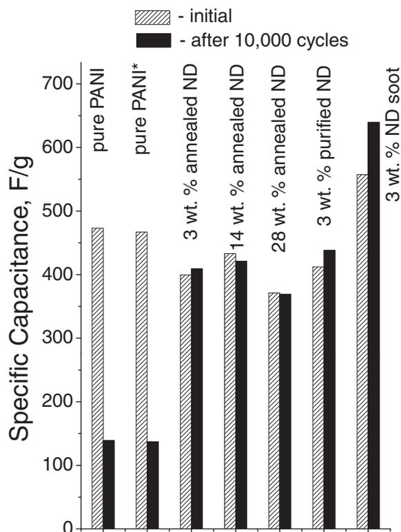
**Figure 5.** Integrated average specific capacitance of the synthesized samples before and after 10 000 cycles. Pure PANI\* sample contains 3 wt% annealed ND mechanically mixed with PANI particles. Other samples contain ND embedded into the PANI particles. The specific capacitance was calculated from the cyclic voltammograms recorded at the sweep rate of  $1 \text{ mV s}^{-1}$  in a symmetric two-electrode configuration.
