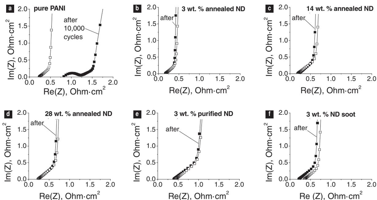
**Figure 6.** Nyquist plots of the PANI-based electrodes: a) pure PANI, b) PANI with imbedded 3 wt% OLC, c) PANI with imbedded 14 wt% OLC, d) PANI with embedded 28 wt% OLC, e) PANI with embedded 3 wt% purified ND, f) PANI with embedded 3 wt% ND soot.
