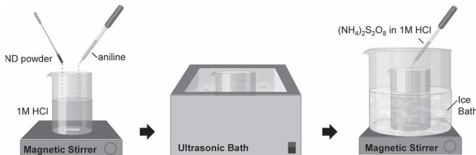
**Figure 1.** Schematic of the PANI and PANI-ND composites' synthesis process.
