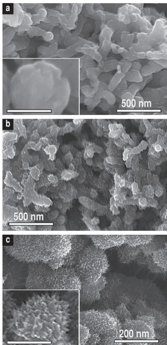
**Figure 3.** SEM images of the synthesized a) PANI and b,c) PANI-ND composite samples. The scale bar in the insets in (a) and (c) is 100 nm.
