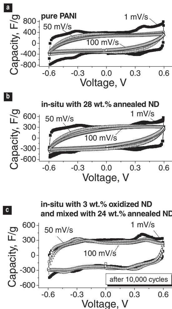
**Figure 7.** CV of the selected PANI-based electrodes recorded at different sweep rates in a symmetric two-electrode configuration: a) pure PANI before long-term cycling, b) PANI with embedded 28 wt% OLC before long-term cycling, c) PANI with embedded 3 wt% purified ND and mixed with 24 wt% OLC after 10 000 cycles.
