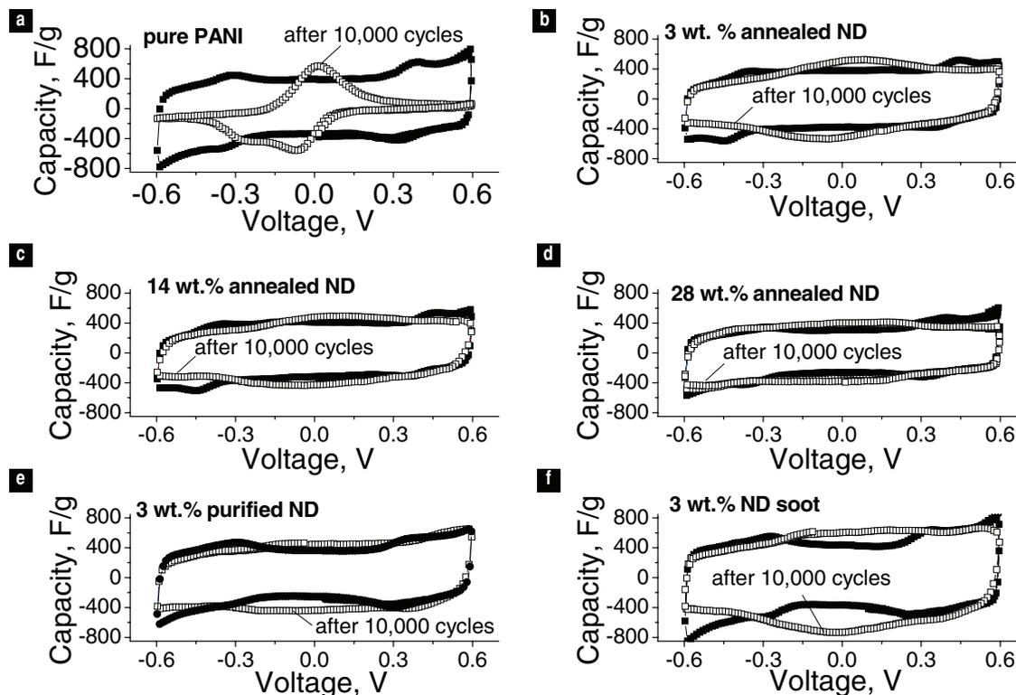
**Figure 4.** CV of the PANI-based electrodes recorded at the sweep rate of  $1 \text{ mV s}^{-1}$  in a symmetric two-electrode configuration before and after 10,000 cycles: a) pure PANI, b) PANI with embedded 3 wt% OLC, c) PANI with embedded 14 wt% OLC, d) PANI with embedded 28 wt% OLC, e) PANI with embedded 3 wt% purified ND, f) PANI with embedded 3 wt% ND soot.
