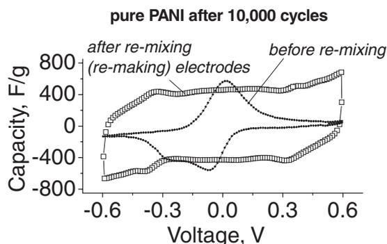
**Figure 8.** CV of the pure PANI electrode recorded at the sweep rate of  $1 \text{ mV s}^{-1}$  in a symmetric two-electrode configuration after 10 000 cycles before and after re-mixing/re-rolling of the electrodes.
