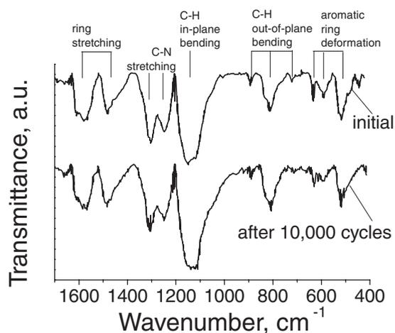
**Figure 9.** Fourier transform infrared spectra of the PANI electrode before and after 10 000 cycles.
