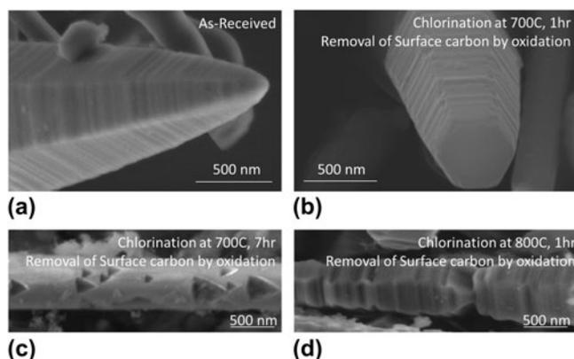
FIG. 6. SEM images of beta-SiC whiskers: (a) as-received and (b–d) after chlorination and removal of the coating by oxidation in air.
