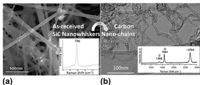
FIG. 8. (a) SEM image and Raman spectrum of as-received SiC nanowhiskers; (b) TEM image and Raman spectrum of nanowhiskers annealed in vacuum at 1700 °C for 30 min.<sup>24</sup>
