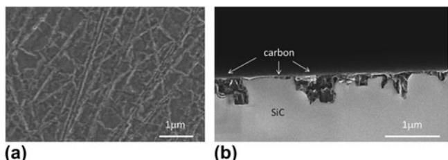
FIG. 2. SEM image of the optical quality polished (000 $\bar{1}$ ) C face of SiC: (a) view from top and (b) from side after vacuum annealing at 1700 °C for 4 h.
