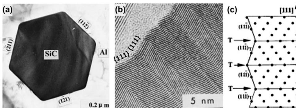
FIG. 7. TEM images of (a) transverse and (b) longitudinal surfaces of the SiC; (c) side surface crystal model of cubic SiC whisker (T denotes twins) (modified from Ref. 23).
