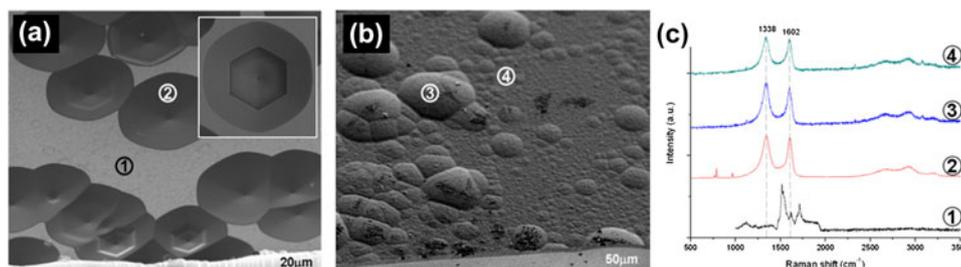
FIG. 5. SEM images of (a) Si and (b) C surface of the 6H single crystalline wafer after chlorination at 1000 °C for 7 h. (c) Raman spectra taken from different regions [as numbered in panels (a) and (b)] of the sample surfaces. (1) From Si face without carbon formation, (2) from Si face inside the hexagonal etch pit, showing carbon formation, and (3, 4) from C face.
