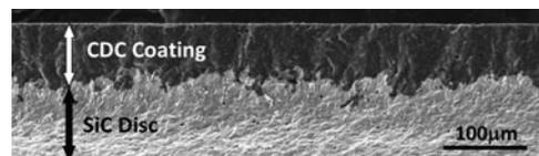
FIG. 1. CDC layer on a sintered SiC polycrystalline ceramic sample produced by chlorination.
