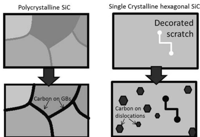
FIG. 9. Schematic showing initial stages of carbon formation on polycrystalline ceramics and single crystal SiC.
