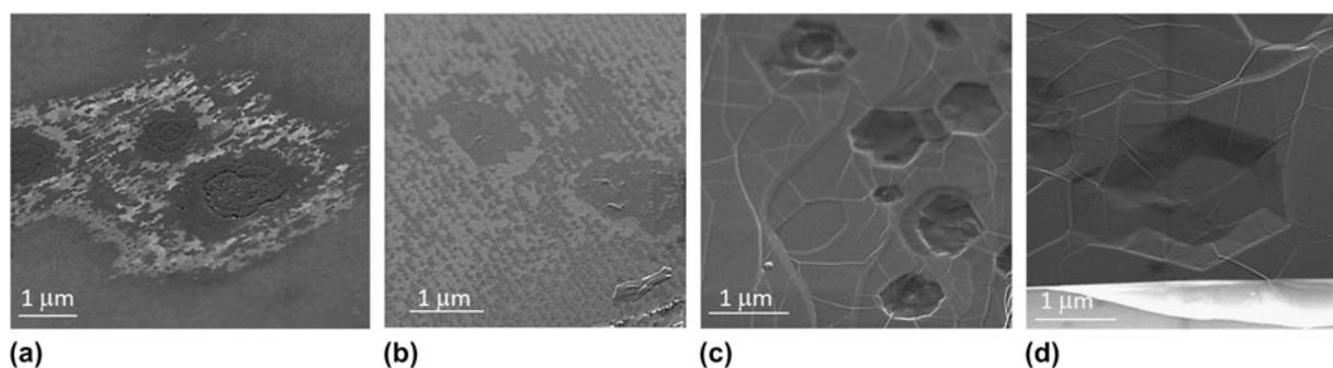
FIG. 3. SEM images of SiC (0001) after vacuum annealing for 4 h at (a) 1400 °C, (b) 1500 °C, (c) 1800 °C, and (d) 1900 °C.
