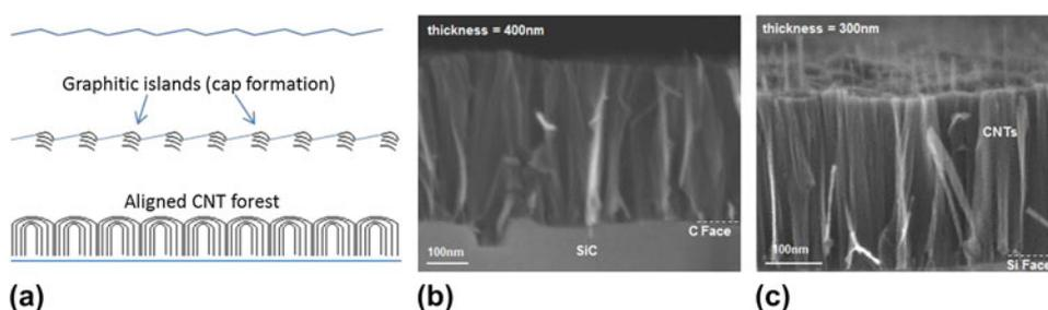
FIG. 4. (a) Schematic illustration; (b, c) SEM images of CNT formation on (b) C face and (c) Si face without pretreatment (b and c are adopted from Ref. 6).
