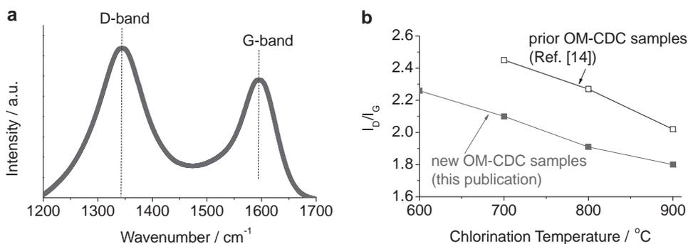
**Figure 2.** Raman spectroscopy studies of OM-CDC: a) a typical Raman spectra of the OM-CDC sample synthesized at 900 °C; b)  $I_{\text{D}}/I_{\text{G}}$  ratio as a function of synthesis temperature.
