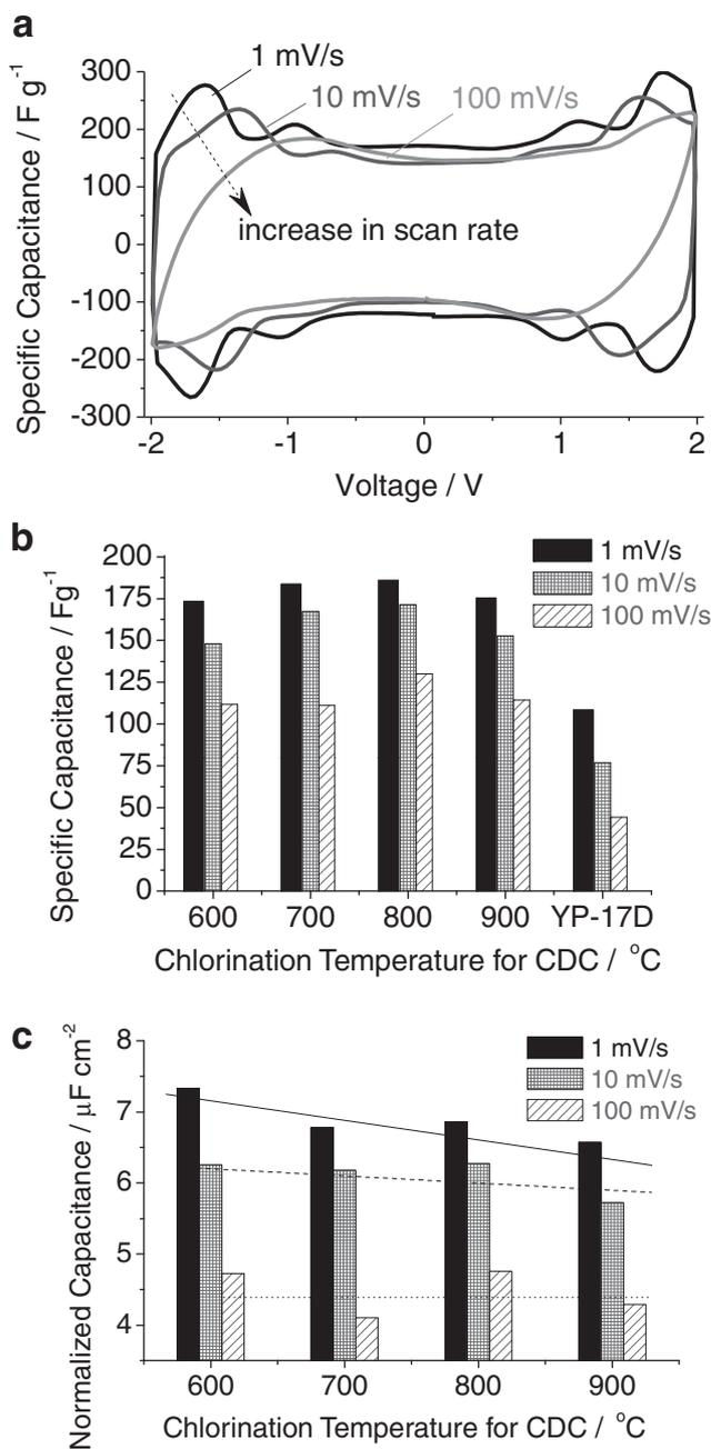
**Figure 3.** Electrochemical characterization of OM-CDC materials in EMIBF<sub>4</sub> ionic liquid at room temperature (20 °C): a) cyclic voltammogram of CDC synthesized at 900 °C; b) specific capacitance of CDC samples at different CV cycling rates in comparison with that of YP-17D activated carbon; c) BET area-normalized specific capacitance as a function of synthesis temperature.
