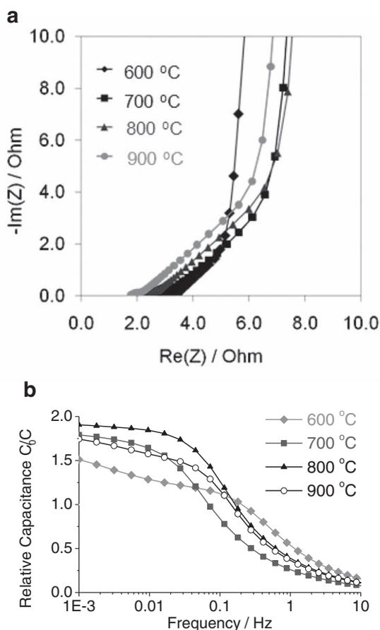
**Figure 4.** Electrochemical characterization of OM-CDC materials synthesized at different temperatures in EMIBF<sub>4</sub> ionic liquid at room temperature (20 °C): a) Nyquist plot, b) frequency response.  $C_0$  in (b) is the specific capacitance of YP-17D measured at 0.001 Hz.
