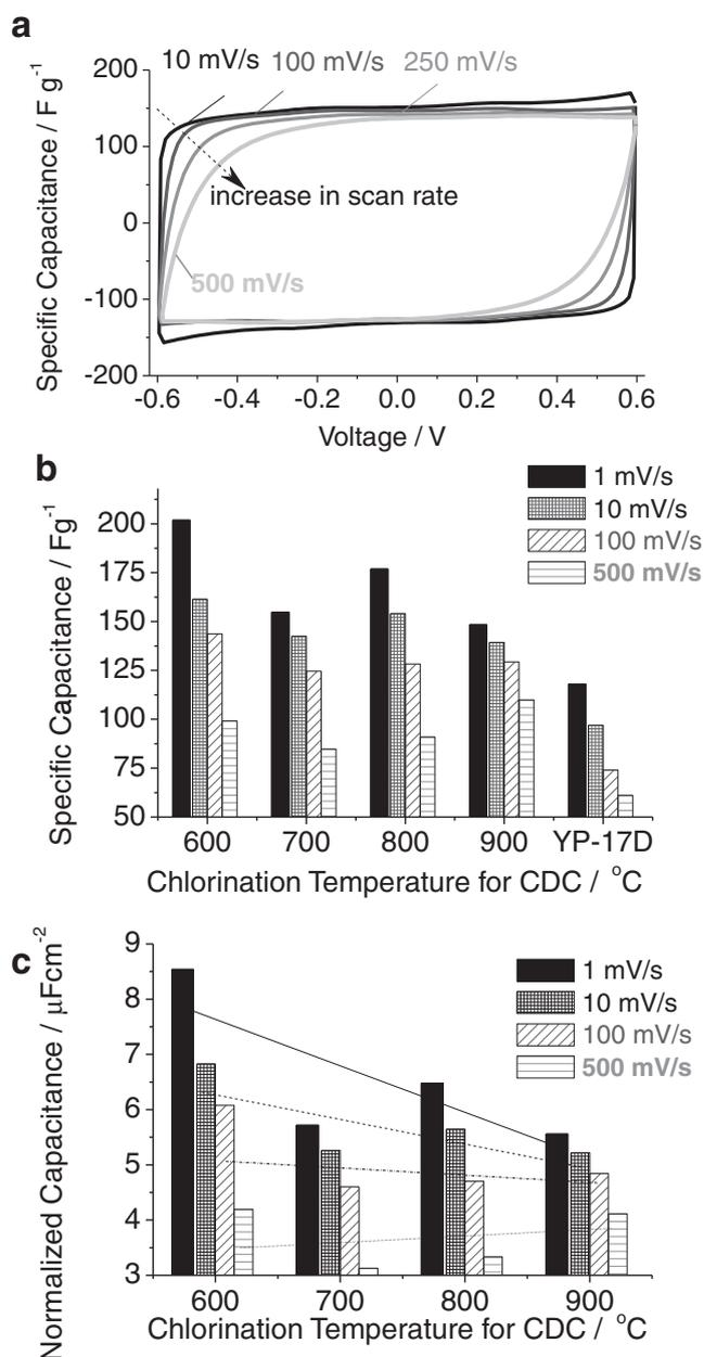
**Figure 6.** Electrochemical characterization of OM-CDC materials in 1 M H<sub>2</sub>SO<sub>4</sub> at room temperature (20 °C): a) cyclic voltammogram of CDC synthesized at 900 °C; b) specific capacitance of CDC samples at different CV cycling rates in comparison with that of YP-17D activated carbon; c) BET area-normalized specific capacitance as a function of synthesis temperature.
