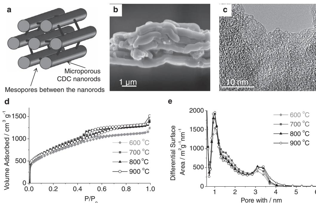
**Figure 1.** Structure and porosity of OM-CDC materials synthesized at different temperatures: a) schematic microstructure; b) scanning electron microscopy (SEM) and c) TEM images showing typical particle morphology and microstructure; d)  $N_2$  gas sorption isotherms; and e) quenched solid density functional theory (QS-DFT) pore size distribution.
