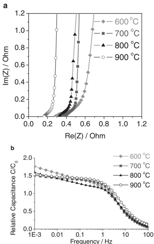
**Figure 7.** Electrochemical characterization of OM-CDC materials synthesized at different temperatures and YP17D in 1 M H<sub>2</sub>SO<sub>4</sub> at room temperature (20 °C): a) Nyquist plot, b) frequency response.  $C_0$  in (b) is the specific capacitance of YP-17D measured at 0.001 Hz.
