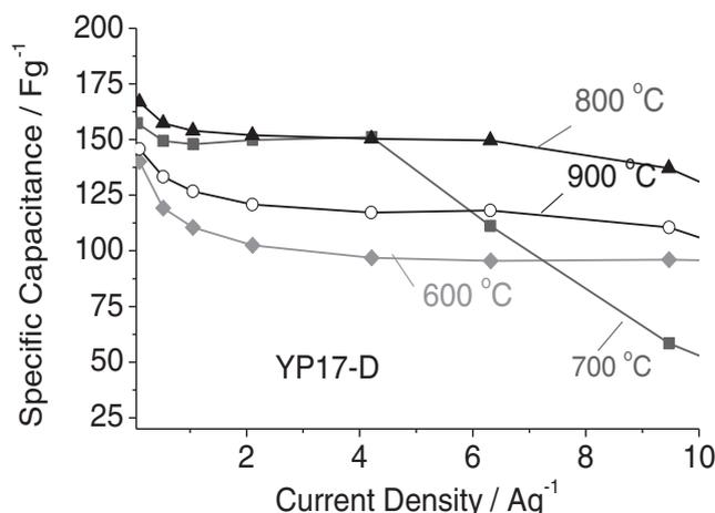
**Figure 5.** Electrochemical characterization of OM-CDC materials synthesized at different temperatures and YP17D in EMIBF<sub>4</sub> ionic liquid at room temperature (20 °C): capacitance retention with current density.
