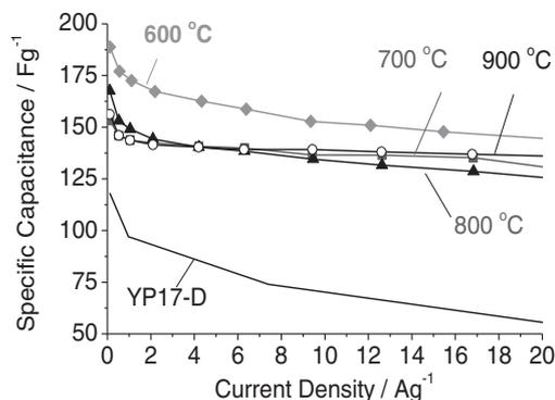
**Figure 8.** Electrochemical characterization of OM-CDC materials synthesized at different temperatures and YP17D in 1 M H<sub>2</sub>SO<sub>4</sub> at room temperature (20 °C): capacitance retention with current density.
