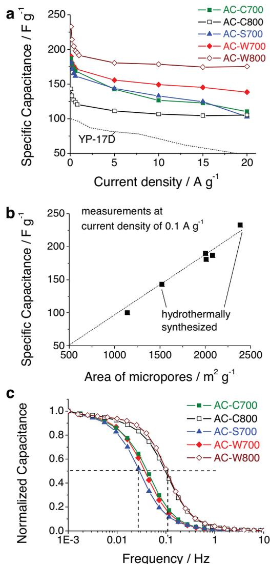
**Figure 4.** Electrochemical characterization of hydrothermally synthesized carbon materials in 1 M tetraethylammonium tetrafluoroborate (TEABF<sub>4</sub>) solution in acetonitrile (AN) at room temperature: a) capacitance retention with current density, b) specific capacitance measured at 0.1 A/g as a function of the NL-DFT specific surface area of micropores, c) frequency response. The performance of commercially available YP-17D activated carbon is provided for comparison.
