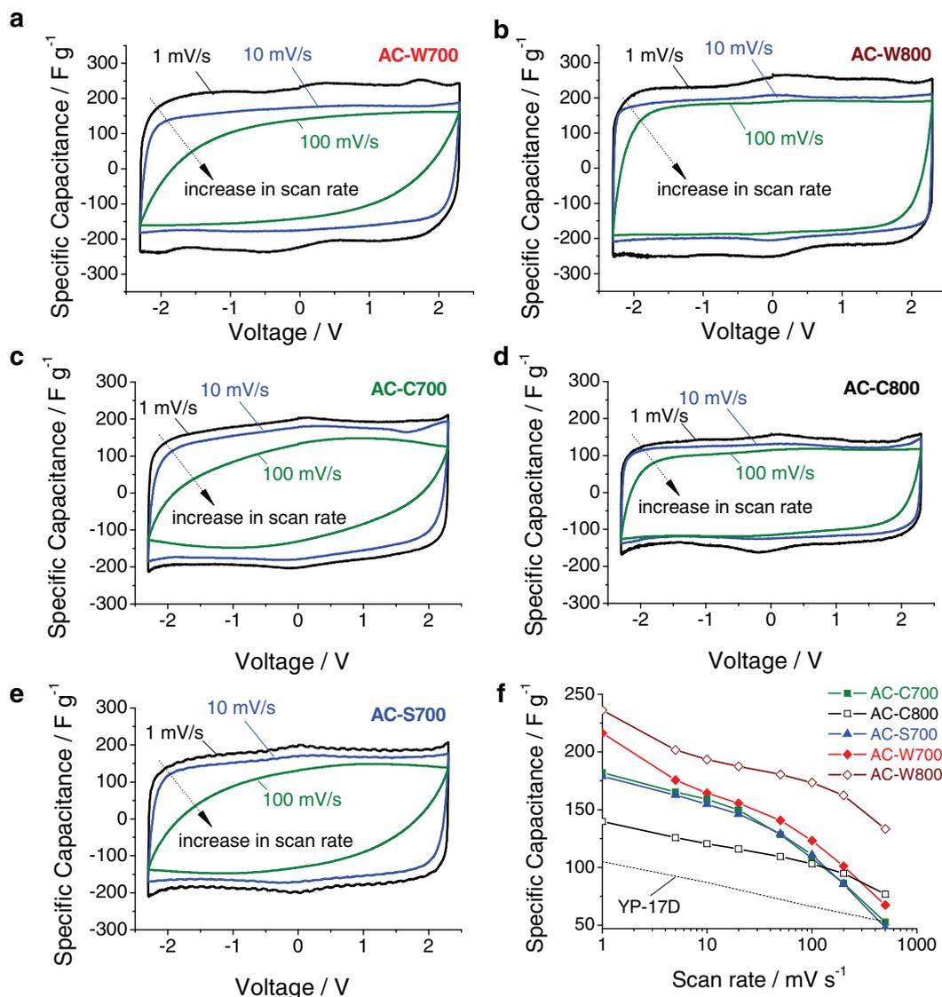
**Figure 3.** Electrochemical characterization of hydrothermally synthesized carbon materials in 1 M tetraethylammonium tetrafluoroborate (TEABF<sub>4</sub>) solution in acetonitrile (AN) at room temperature: a–e) cyclic voltammograms (CV) of the carbon samples; f) specific capacitance of carbon samples at different CV scan rates in comparison with that of commercially available YP-17D activated carbon.
