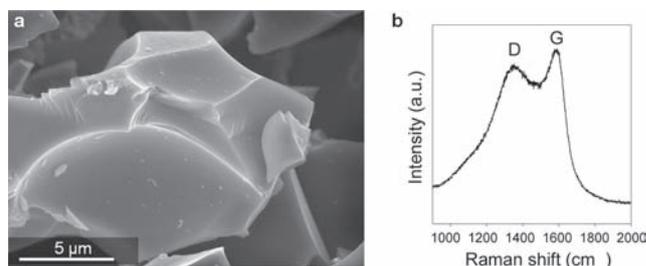
**Figure 1.** Structure of the microporous carbon materials produced by hydrothermal carbonization: a) a scanning electron microscopy (SEM) image showing typical particle morphology; b) a typical Raman spectra of synthesized carbons.
