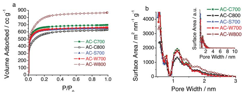
**Figure 2.** a)  $N_2$  adsorption/desorption isotherms and b) pore size distribution (PSD) for hydrothermally synthesized carbons after activation. The PSD was derived from the  $N_2$  isotherms using non-local density functional theory (NL-DFT). The inset in (b) shows the complete lack of pores  $>3$  nm in these carbons. The dip in the PSD at 0.9 nm is an artifact of the calculations.
