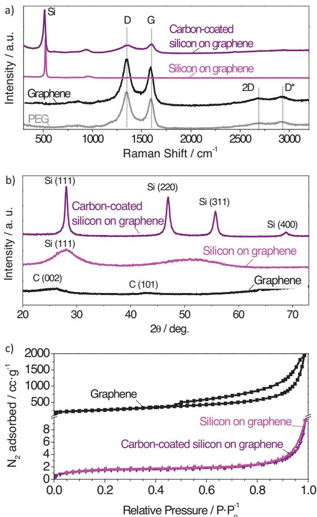
**Figure 3.** Characterization of the graphene and graphene-based materials by a) Raman spectroscopy, b) X-ray diffraction and c)  $N_2$  physisorption.
