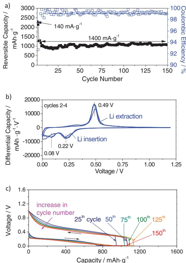
**Figure 4.** Electrochemical performance of the C-Si-graphene electrode: a) capacity (per mass of the composite) and Coulombic efficiency as a function of cycle number, b) a differential capacity plot and c) charge-discharge profiles for selected cycles.
