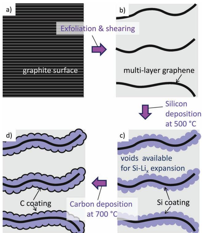
**Figure 1.** Schematic of C-Si-graphene composite formation: a) natural graphite is transformed to b) graphene and then c) coated by Si nanoparticles and d) a thin C layer.
