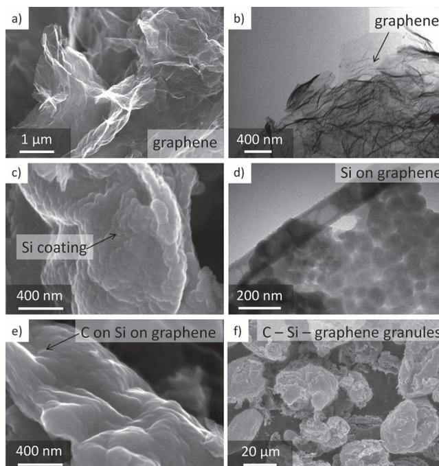
**Figure 2.** Structure of the Si-graphene materials. a, c, e, f) SEM and b, d) TEM micrographs of a, b) graphene, c, d) Si-coated graphene, and e, f) C-Si-graphene granules.
